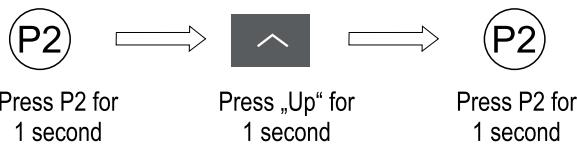
Press whether the „Up“ or the „Down“ button for a short movement - corresponds 10° - (let go within 2 seconds), if that button is being pressed longer than 2 seconds, the motor will move continuously.
