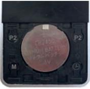
The access to the battery compartment is at the back of the emitter (see illustration on the left). Simply push the battery compartment cover downwards. The used button cell can now be removed and replaced.
