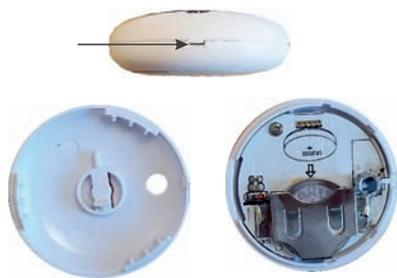
When the battery is low, the LED will flash 10 times every 2 minutes. In this case, immediately replace the battery of the sun sensor. Access to the battery compartment is located on the side of the sun sensor (see illustration on the left). Open the cover with a suitable tool. The used button cell can now be removed.
