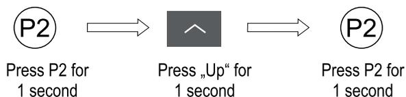
Press whether the „Up“ or the „Down“ button for a short movement - corresponds 10° - (let go within 2 seconds), if that button is being pressed longer than 2 seconds, the motor will move continuously.
