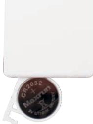
The access to the battery compartment is located at the bottom of the emitter (see illustration on the left). There is a small gap between the battery compartment cover and the housing. Use a suitable tool to carefully remove the battery compartment cover. The battery compartment can now be completely opened by a rotary movement. The used button cell can now be removed.
