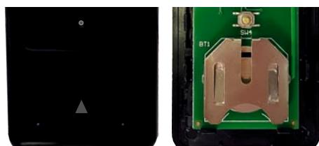
The access to the battery compartment is at the back of the emitter (see illustration on the left). Simply push the battery compartment cover upwards. The used button cell can now be removed and replaced.
