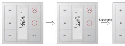
Press "Up" and "Stop" button simultaneously and hold for 6 seconds.
