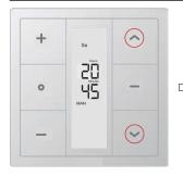
Press "Up" and "Stop" button simultaneously and hold for 6 seconds.
